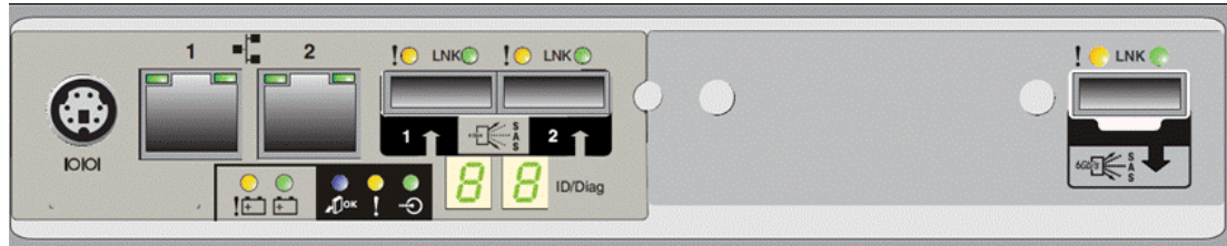
Figure 4-1 The rear panel of a DS3500 controller
