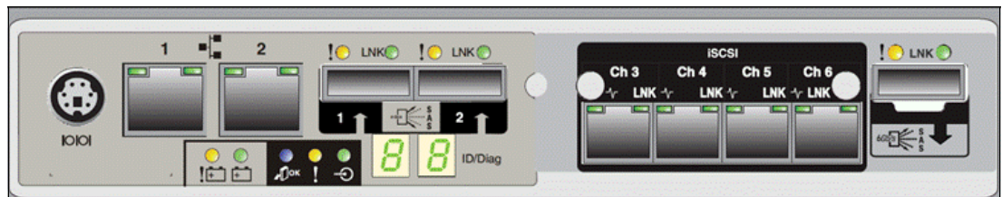
Figure 2-8 Controller module with optional iSCSI host interface daughter card
