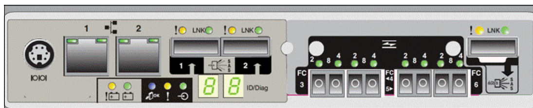
Figure 4-3 The rear panel of a DS3500 controller with the optional Fibre Channel host port adapter installed
