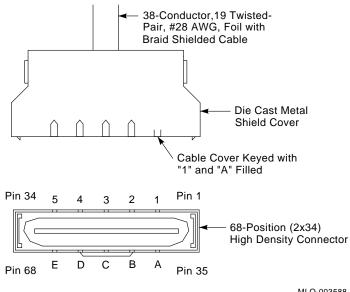
The shielded 68-pin connector ( Figure 1–9) for the 68-pin to 50-pin adapter cable consists of two rows of contacts spaced 5.51 mm (.217 in) apart.
