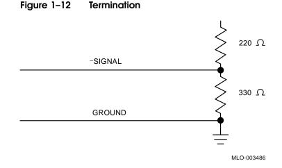
Near-end termination is provided within the system enclosure. The far-end termination for the external bus is provided by a terminator plugged into the last SCSI device connector. There must be no other terminators on the bus. The bus must be terminated externally. If you follow these rules for all devices, you will be able to configure the bus with proper termination.
