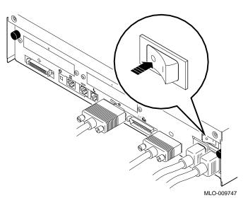
Figure 2–5 Turning Off the System Unit
