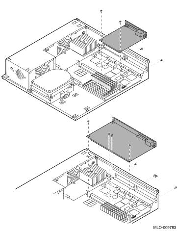
Figure 2–23 Removing and Installing a TURBOchannel Option
