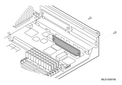
Removing and Installing a TURBOchannel Option (For Models 300/300X/300LX Systems)
