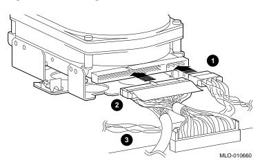
Cabling for Drive in Position 2 To cable the drive that you are installing in position 2, follow these steps and refer to Figure 2-18:
