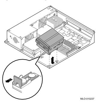
Figure 2–11 Removing a Removable-Media Drive
