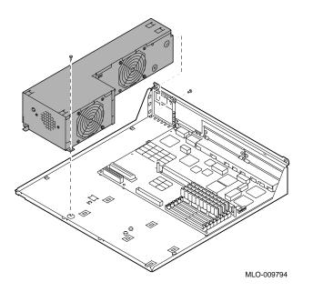
**Caution: Shield** It is possible for the metal shield that is attached to the inside of the system unit to come loose when you remove the power supply. This shield is located at the back of the system unit and encircles the opening through which the power supply sockets extend (see Figure 2–28). If the shield comes loose, be sure to reinstall it.
