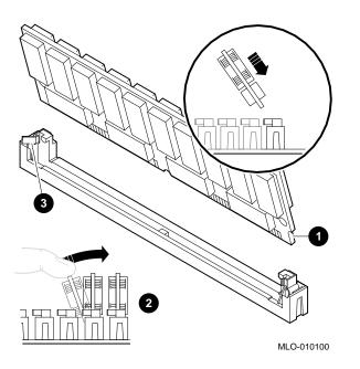
**Install Memory** To install memory, reverse the steps in the removal procedure, as follows, and refer to Figure 2–22:
