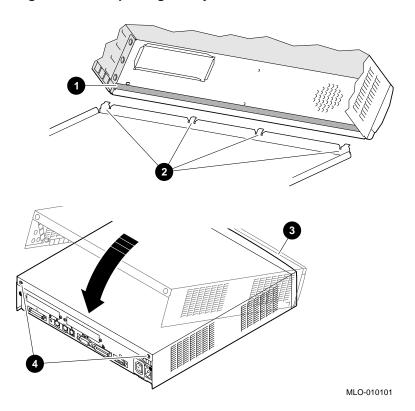
Figure 2–31 Replacing the System Cover
