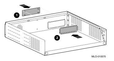
Remove the Filler Panel and Metal Shield If you did not order a removable-media drive from the factory when you placed your order with Digital, and are installing one now, you must first remove the plastic filler panel and metal shield from the front bezel on the system unit cover.
