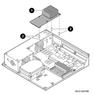
Figure 2–25 Removing the CPU Module
