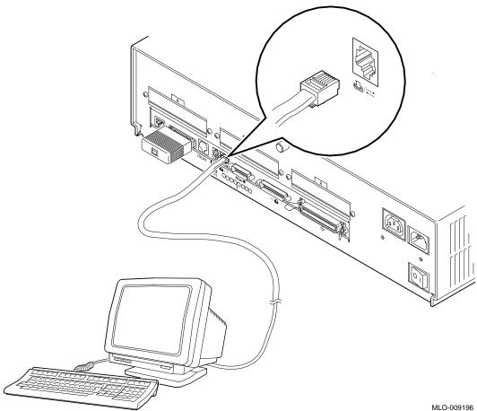
Check the Alternate **Console Switch**  If you connected a terminal to use as an alternate console device (Step 2), you should check to make sure that the alternate console switch is in the correct position.
