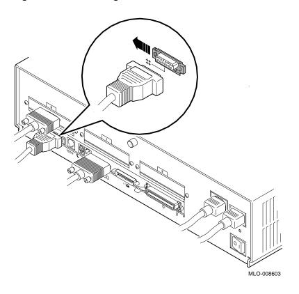
Figure 5-1 Connecting to an AUI Ethernet Network
