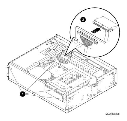
Moving the Secure System Jumper
