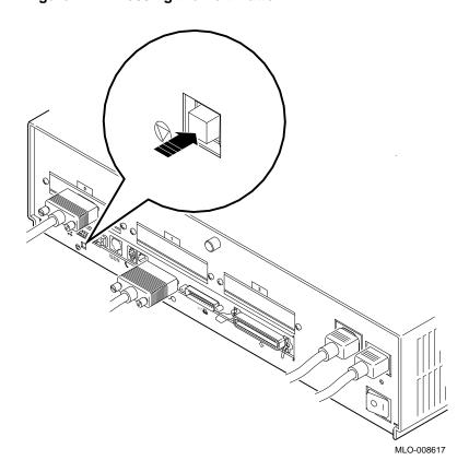
Figure 7–2 Pressing the Halt Button
