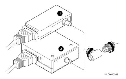
Step 5: **Terminate** Connection If your workstation is the last one on a ThinWire network, you need to terminate the network connection. Do this by connecting a terminator, rather than a ThinWire network cable, to one side of the T-connector connected to either the DECXM Transceiver **1** (or the DESTA unit **2**), as shown in Figure 5–5.
