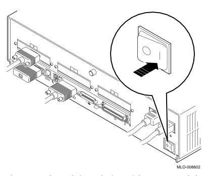
Figure 6-1 Turning On the DEC 3000 Model 400/400S AXP **System**
