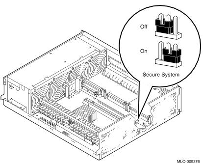
Moving the Secure System Jumper
