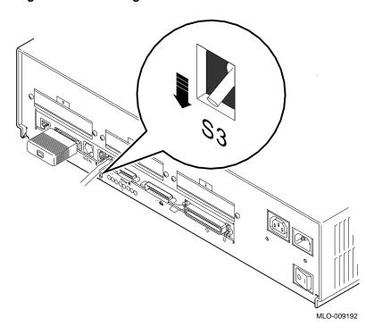
Figure 4–4 Checking the Alternate Console Switch
