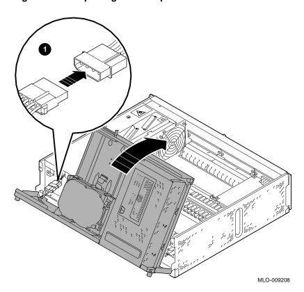
Figure 11-5 Replacing the Driveplate
