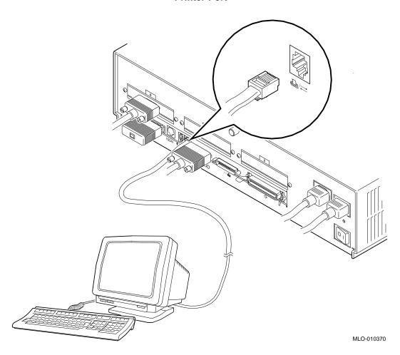
Step 2: Change the Alternate **Console Switch**  The alternate console switch on the rear of the system unit directs console output to one of two destinations: a monitor or an alternate console device, such as a terminal or a printer.
