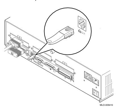
Modem Loopback Connector If your Digital service representative requests that you connect the modem loopback connector, connect it as shown in Figure 14–9.
