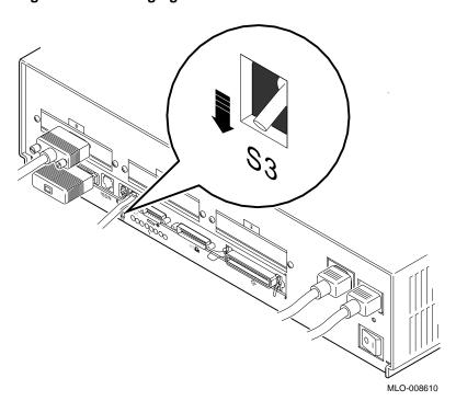
Figure 12–2 Changing the Alternate Console Switch
