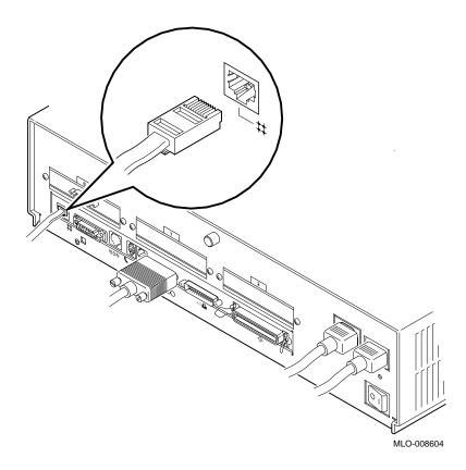
Figure 5–2 Connecting a 10BASE-T Network Cable
