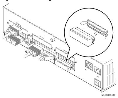
Figure 14–10 Connecting the SCSI Terminator
