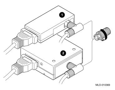
Figure 5–5 Terminating the Ethernet Connection
