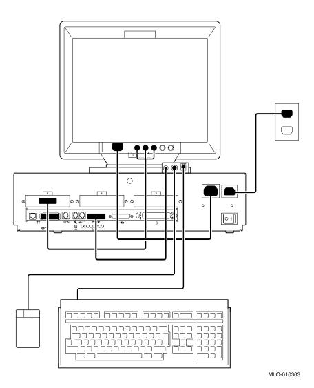
Figure 3–10 A Connected Workstation
