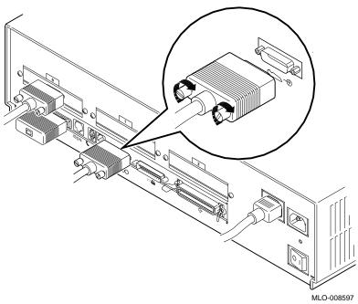
Step 8: Keyboard and **Mouse Cables** to Extension Cable
