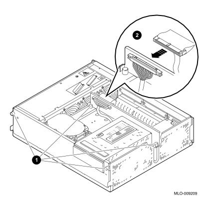
Moving the Secure System Jumper
