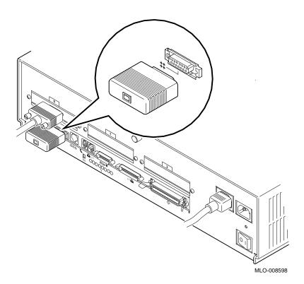
Step 7: Keyboard/Mouse Cable to System Unit
