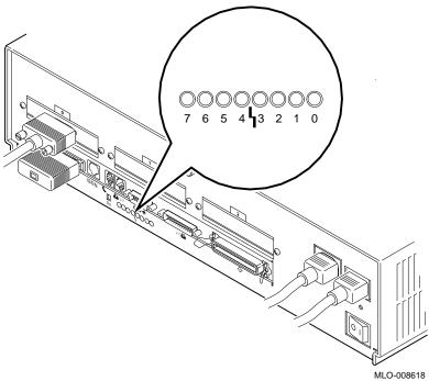
The diagnostic display lights can provide your Digital service representative with important information in determining the source of a problem.
