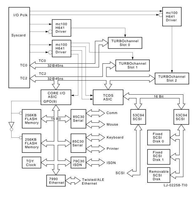
Figure 1–2 DEC 3000 Model 400/400S System I/O Subsystem Block Diagram
