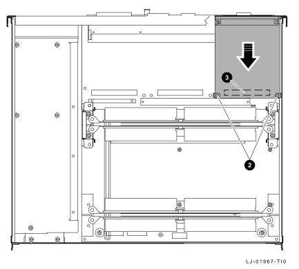
Figure 7–17 Removing the TURBOchannel Option
