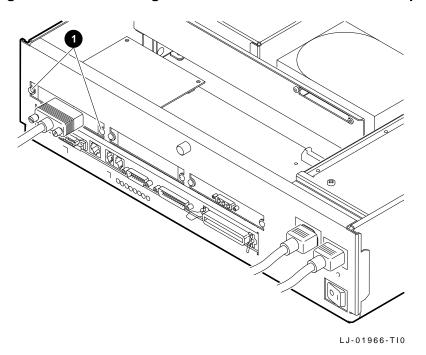
Figure 7–16 Removing the Screws from TURBOchannel Option
