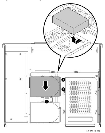
Figure 7–11 Removing the Fixed Media
