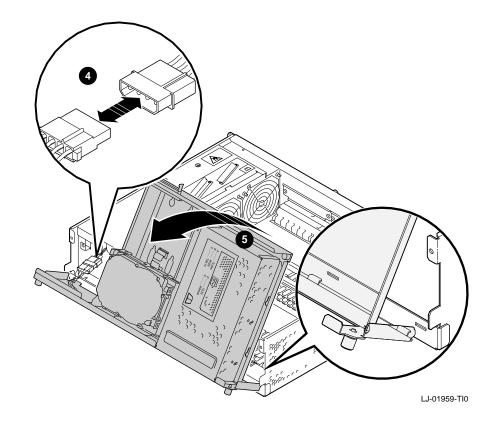
Figure 7–15 Removing the Drive Shelf
