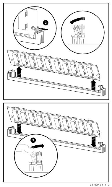
Figure 7–19 Removing the SIMMs
