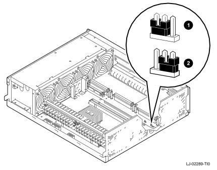
In the enabled position, the ROM can be rewritten when new versions of the firmware are distributed.
