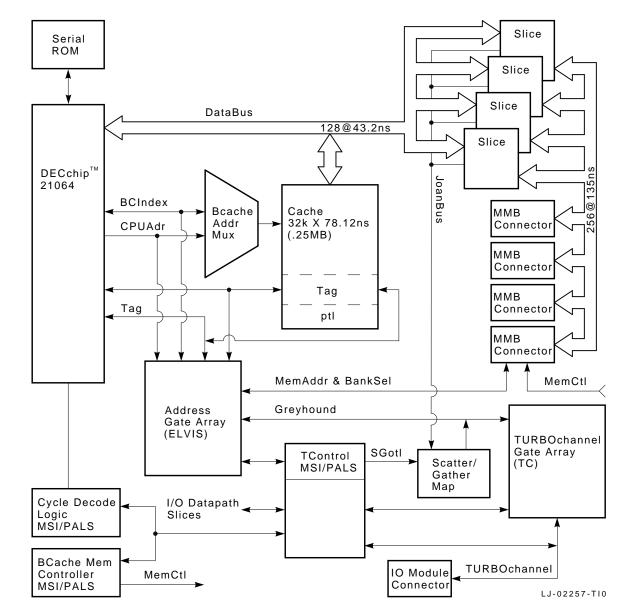
Figure 1–1 DEC 3000 Model 400/400S AXP system Module Block Diagram
