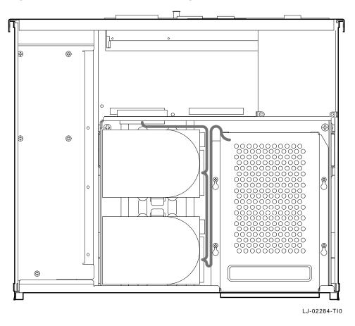
Figure 7–4 Disk SCSI Cable Routing
