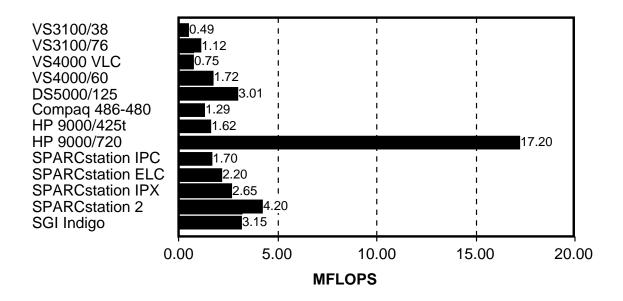
Figure 4-12: Linpack Double Precision MFLOPS Ratings
