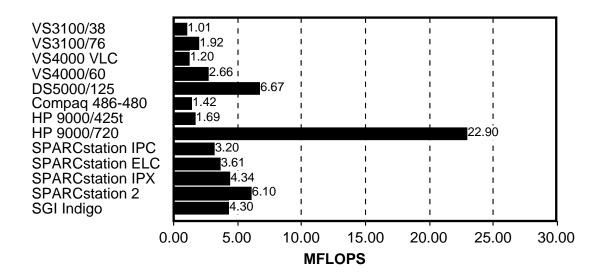
Figure 4-11: Linpack Single Precision MFLOPS Ratings
