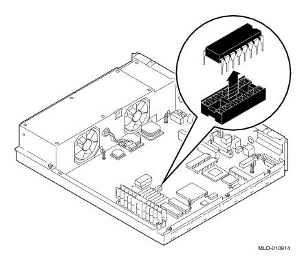
Set the Ethernet ROM on an antistatic mat until you are ready to install it in the VAXstation 4000 system.
