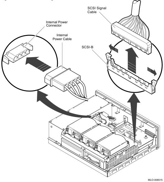
Figure 3–2 Disconnecting the SCSI and Power Cables
