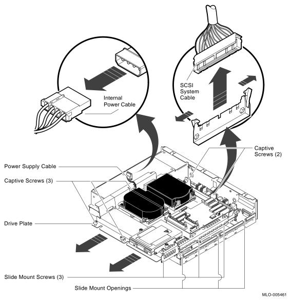
5. Loosen the five captive screws and the three Phillips-head slide mount screws on the drive plate. Do not remove the screws.
