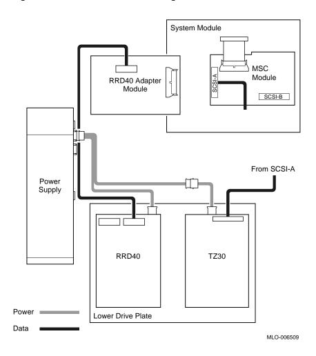
Figure 3–5 Lower Drive Plate Configuration
