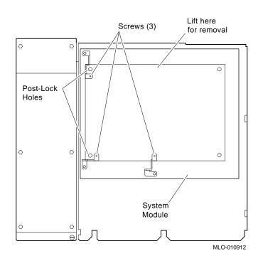
Figure 4–5 Scanline Coprocessor Mounting Brackets
