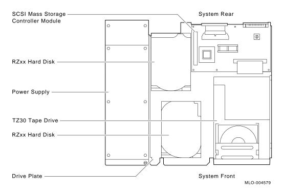
**Remove RZ2x**Remove all the supported RZ2x disk drives from the drive plate.**Disk Drives**Two of these drives can be installed into the VAXstation 4000<br/>system unit.
