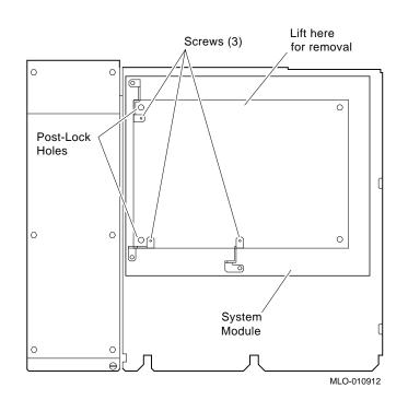
Figure 3–7 Scanline Coprocessor Mounting Brackets
