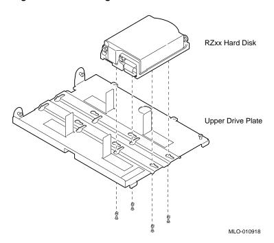
Figure 3–4 Removing RZ2x Fixed Disks from the Drive Plate
