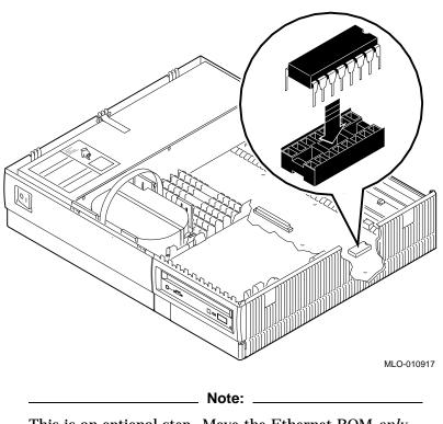
This is an optional step. Move the Ethernet ROM *only* if you want to maintain the same VAXstation 3100 Ethernet address in the VAXstation 4000 system.
