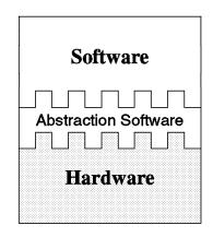
Figure 3. PReP Specification Compatibility Model. Abstraction layer separates hardware and software.
