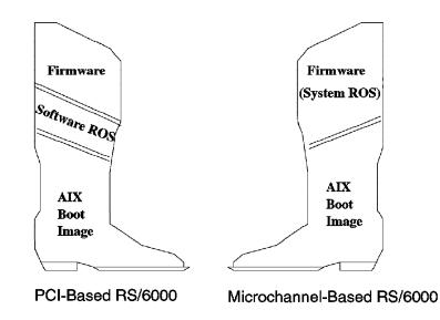
Figure 16. Boot Structure on PCI-Based RS/6000 Systems and Microchannel-Based RS/6000 Systems
