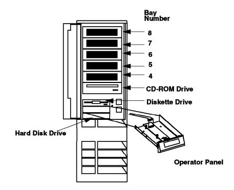
Figure 9. RS/6000 Model E20 Front View
