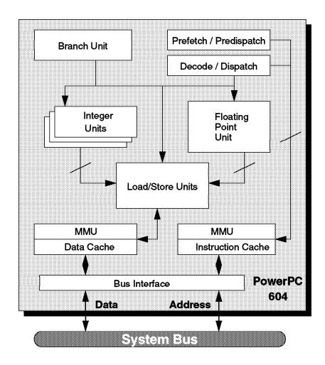
Figure 6. PowerPC 604 Microprocessor Logical Block Diagram
