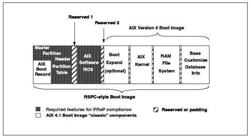
Figure 22. Boot Image Layout on PCI-Based RS/6000 Systems
