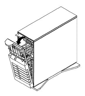
Figure 14. Removing the Front Panel
