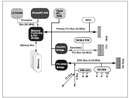
Figure 5. PCI RS/6000 Entry Server Logical Block Diagram
