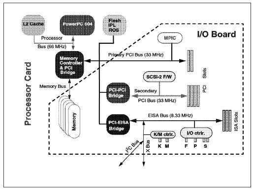
Figure 7. PCI-Based RS/6000 Server's Electronics Partitioning
