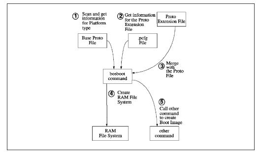
Figure 21. Relation Map of Base Proto and Proto Extension Files
