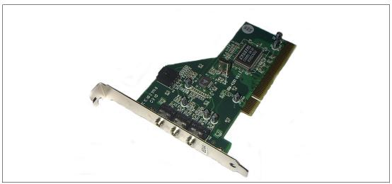
Figure 2-9 PCI audio adapter
