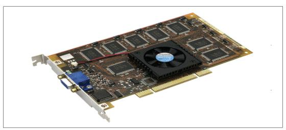
Figure 2-6 The GXT135P graphics accelerator
