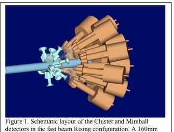
diameter beam pipe passes through the array.
